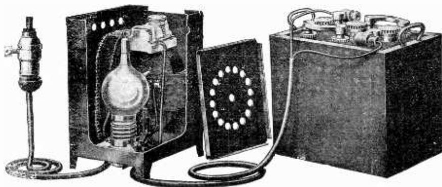
Schematic view of the Tungar apparatus connected up to AC Supply and arranged to deliver accumulator charging current.
